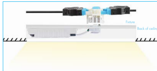
Install to luminaires to achieve easy extension
